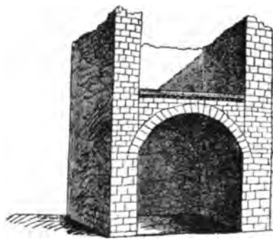
FLOORING OVER AN ARCHED ROOM
